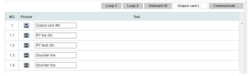
The output card (4M) has four configurable outputs. The default settings for the outputs are:
